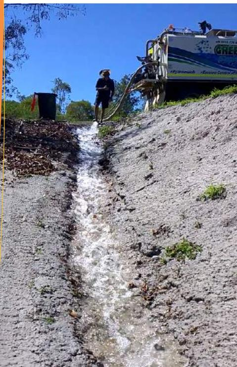
Resistance to erosion by surface flow would be comparable to cement based coatings ...
